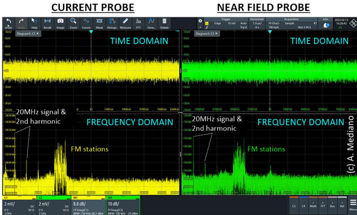
Please take note that the analog signal is present in cable 1, whereas our measurement is being conducted on cable 4. This discrepancy arises from the occurrence of crosstalk between cables. To confirm the absence of signal detection by the probes, we performed a null experiment.
