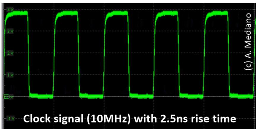
*Fig. 6.- Clock signal in cable 5.*
