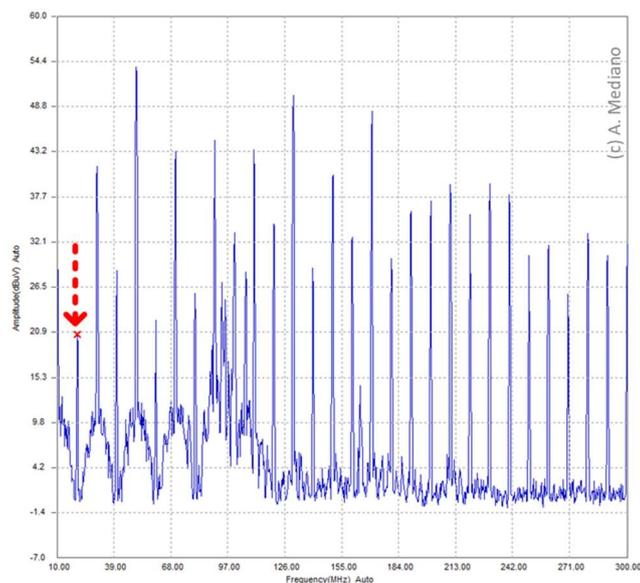
Fig. 15.- With a click of the mouse we can ask for the frequency of interest.
