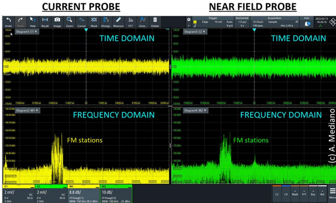
Observe how FM broadcasting stations are detected due to the cable functioning as a receiving antenna. While this effect can be mitigated by conducting measurements in a shielded tent, such measures are often unnecessary for many debugging tasks.
