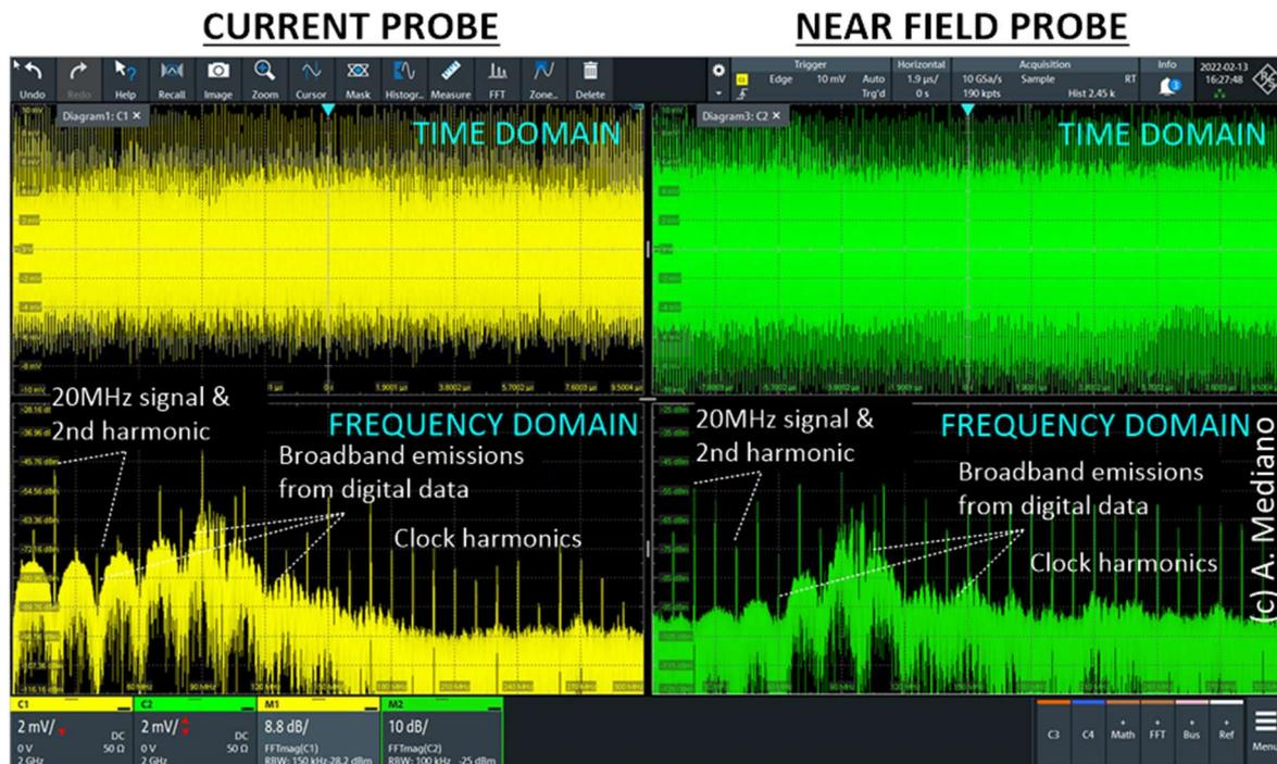
Fig. 11.- Measurements when analog signal (cable 1), data (cable 4), and clock (cable 5) are activated in System 1.
