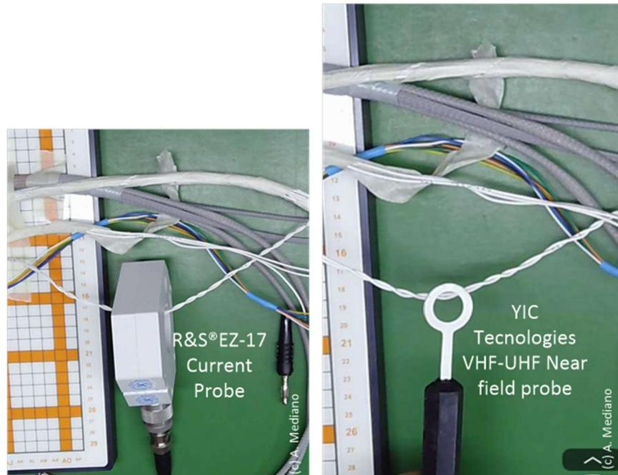
*Fig. 7.- Testing the twisted pair with current probe and near field probe.*
