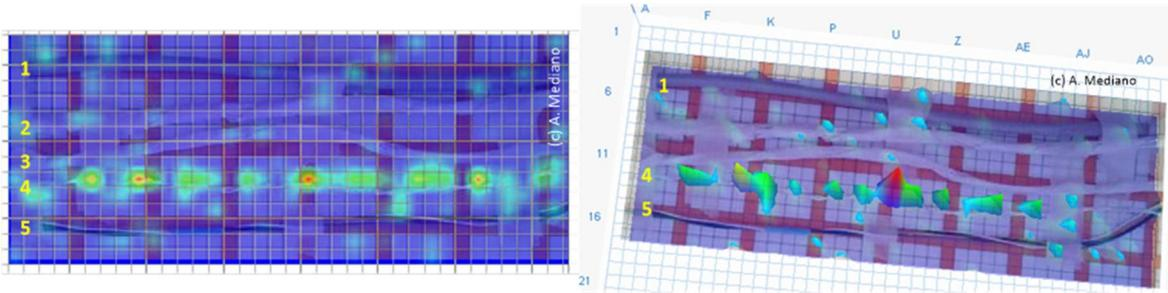
Fig. 18.- The energy from digital data is clearly located around cable 4.
