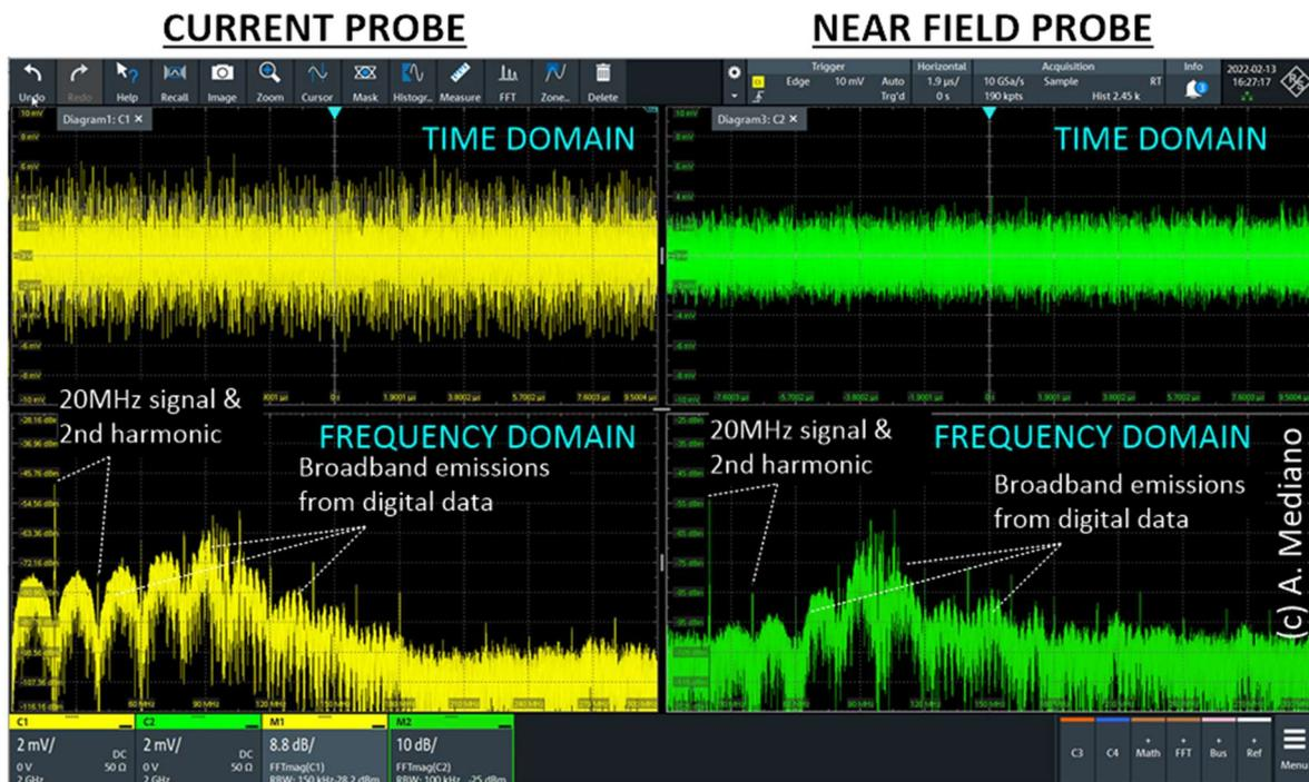
Fig. 10.- Measurements when the analog signal (cable 1) and data (cable 4) are activated.
