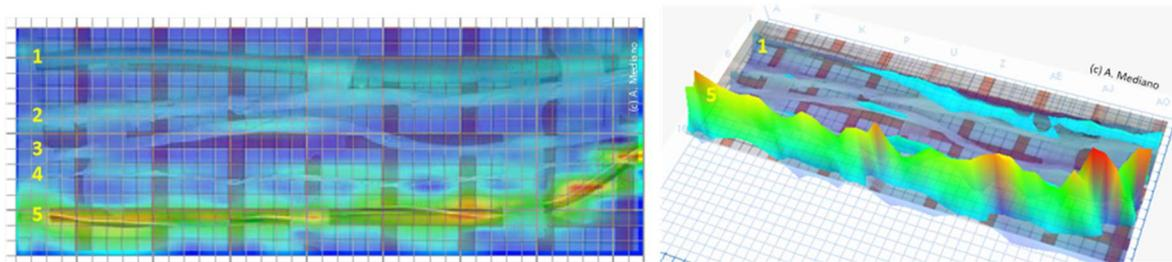
Fig. 14.- With the used scale we can see that maximum amplitudes are detected in cable 5.
