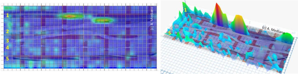
Fig. 16.- Where the 20MHz energy is detected. Basically, in cable number 1 but note second harmonic in 10MHz clock signal (cable 5) has some contribution for energy in that frequency.
