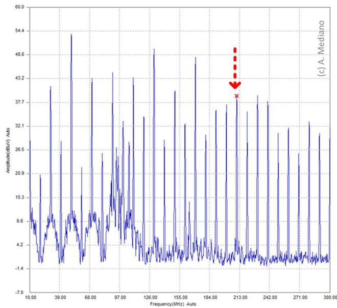
Fig. 19.- How to specify interest to locate where 210MHz energy is located (21th clock harmonic).
